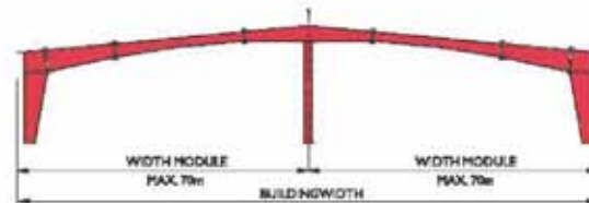
MULTISPAN "1" (MS-1) (1 Interior Column)
